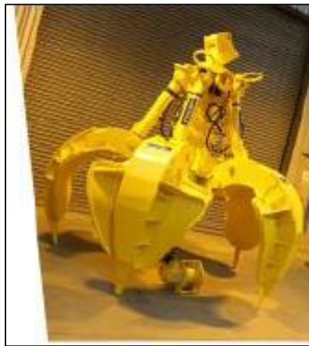
Figure 14: Example grab attached at the end of the crane.
