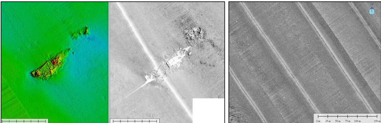
Figure 9: Typical Multibeam and side scan sonar imagery, showing a wreck with debris (left) and boulders (right).
