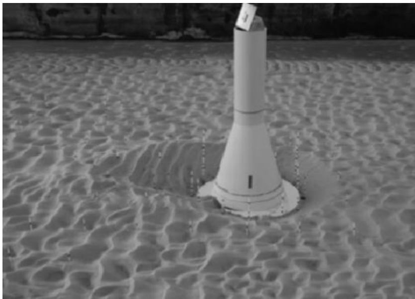
Figure 6: Form of the equilibrium scour hole developed around a conical GBS foundation in a scaled model test for Thornton Bank (Bolle et al., 2010).
